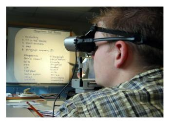
A video magnifier is a system that uses a video camera to project a magnified image of printed text, handwriting or photographs onto a video monitor, PC or TV screen. Some video magnifier models (e.g. room viewing systems) have the capability to view the blackboard or materials posted on walls around the classroom.
