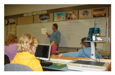
A video magnifier is a system that uses a video camera to project a magnified image of printed text, handwriting or photographs onto a video monitor or TV screen. Some video magnifier models (e.g. room viewing systems) have the capability to view the blackboard or materials posted on walls around the classroom.
