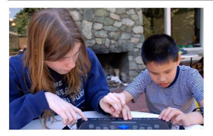
A refreshable Braille device is an electromechanical device for displaying Braille characters, usually by means of raising dots through holes in a flat surface. These displays can be attached to a computer or integrated into a Braille Notetaker.
